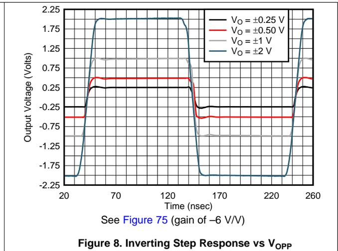
Figure 8. Inverting Step Response vs  $V_{OPP}$
