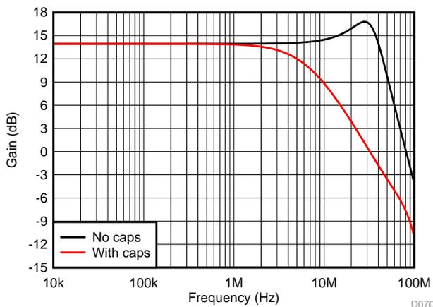
Figure 65. Inverting Response With and Without Compensation
