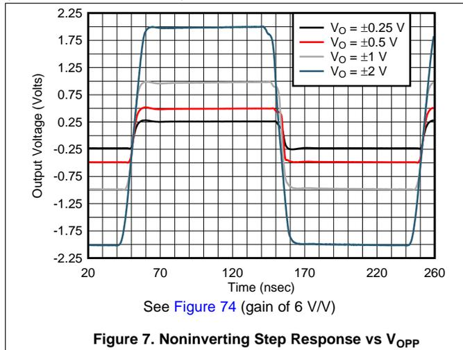
Figure 7. Noninverting Step Response vs  $V_{OPP}$
