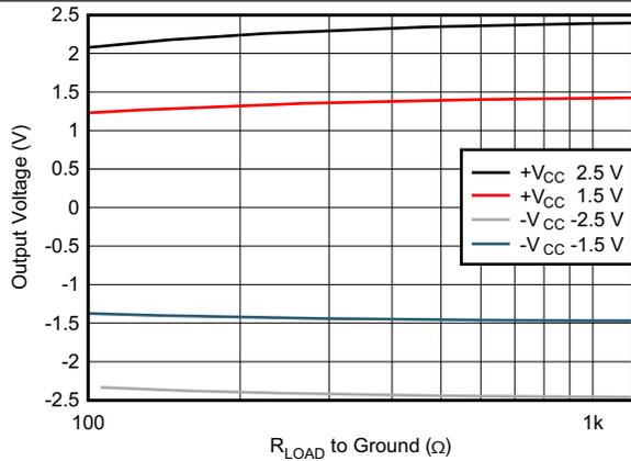
Figure 55. Output Voltage Swing vs Load Resistor
