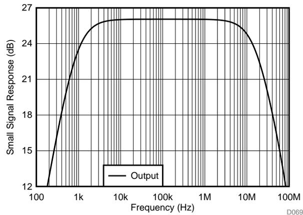
**Figure 73. Inverting Single-Supply Response With AC-Coupled Input**
