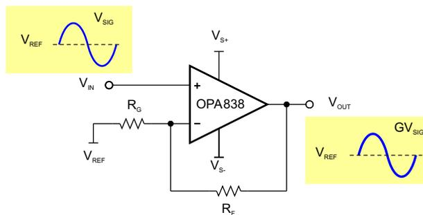
Figure 61. Noninverting Amplifier
