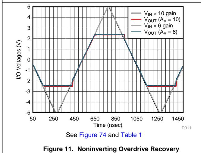
Figure 11. Noninverting Overdrive Recovery
