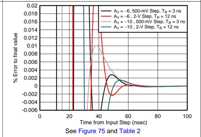
Figure 10. Simulated Inverting Settling Time
