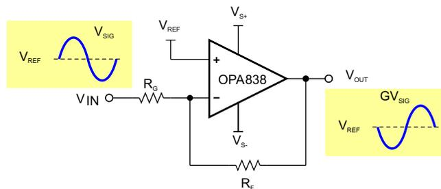
Figure 62. Inverting Amplifier
