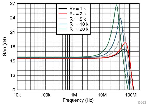
Figure 63. Frequency Response With Various Feedback Resistor Values
