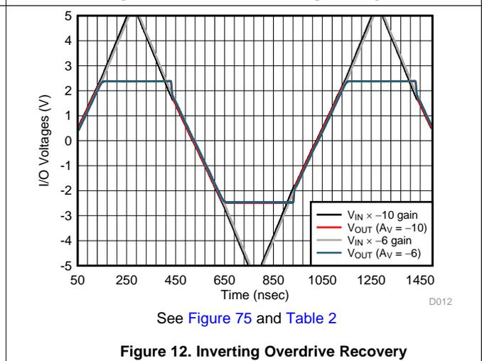
Figure 12. Inverting Overdrive Recovery
