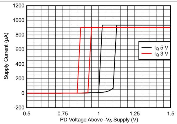
Figure 58. Supply Current vs Power-Down Voltage: Turnon Higher Than Turnoff
