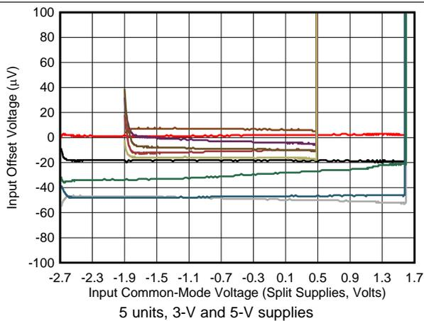
Figure 59. Input Offset Voltage vs Input Common-Mode Voltage
