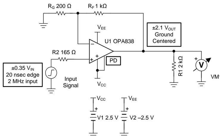
Figure 68. Split-Supply Operation
