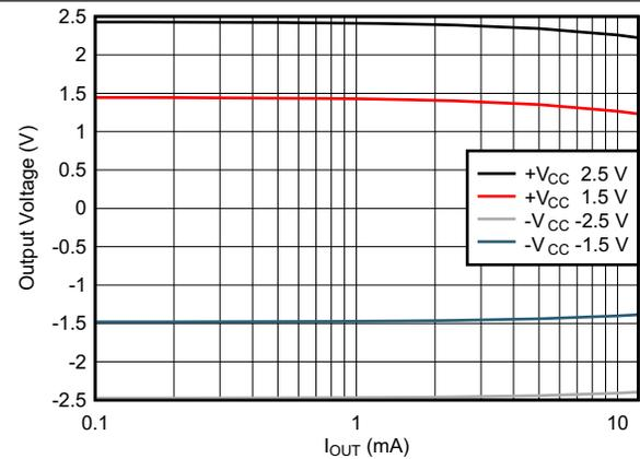
Figure 56. Output Saturation Voltage vs Load Current
