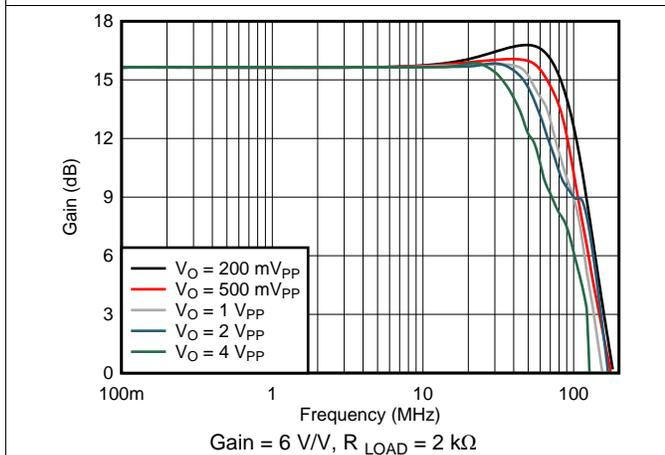
Gain = 6 V/V,  $R_{LOAD} = 2\text{ k}\Omega$
