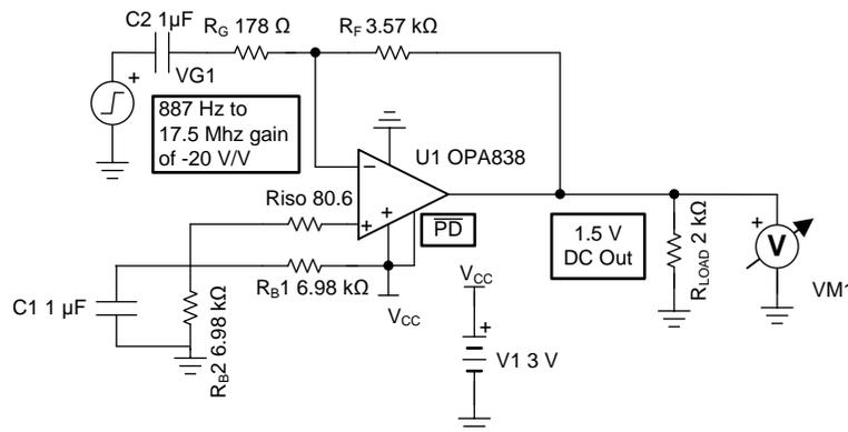
Figure 72. Single-Supply Inverting Gain Stage With AC-Coupled Input
