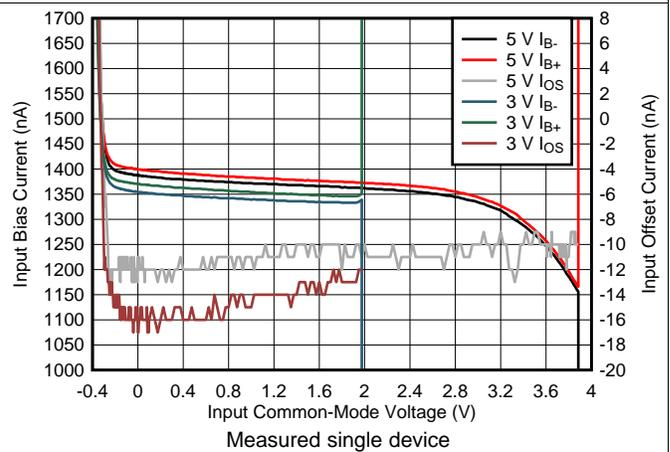
Figure 60. Input Bias and Offset Current vs  $V_{ICM}$
