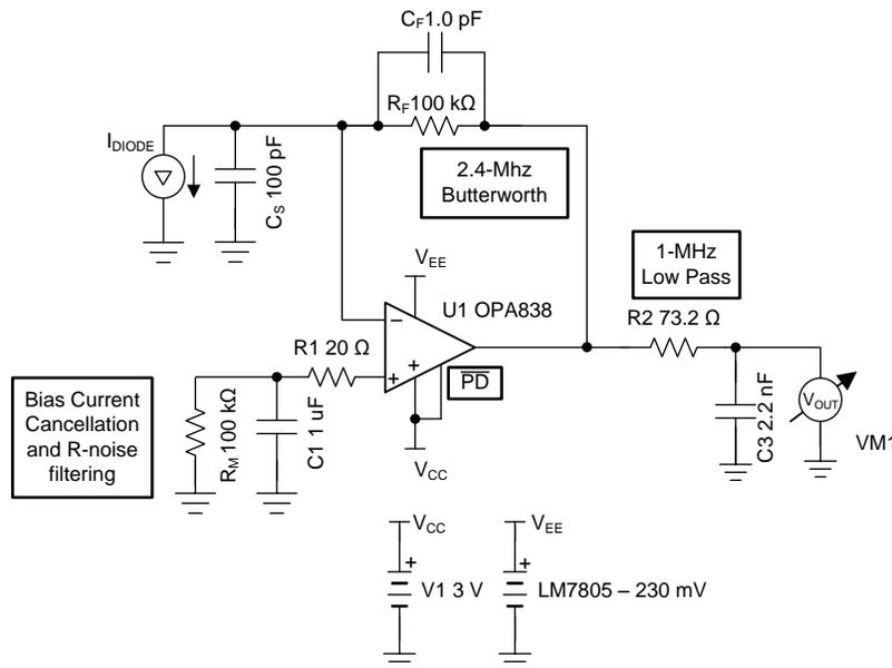
**Figure 80. 100-k $\Omega$  Wide Bandwidth Transimpedance Design**
