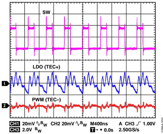
Figure 23. Typical Switch and Voltage Ripple Waveforms in Cooling Mode  $V_{IN} = 3.3V$ , Load =  $2\Omega$ , TEC Current = 1A
