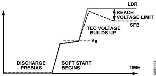
Figure 30. Soft Start Profile in Cooling Mode
