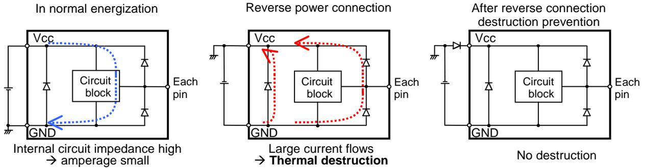
Fig.16 Current flow when power is connected reversely
