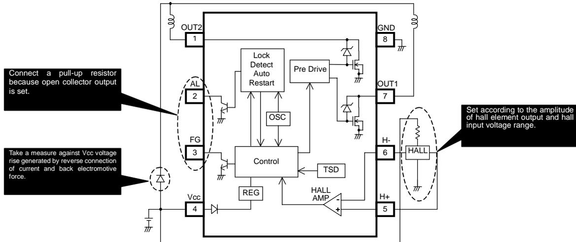
Fig.12 application circuit
