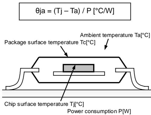
Fig.14 Thermal resistance
