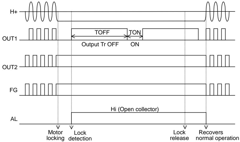
Fig.13 Lock protection (incorporated counter system) timing chart
