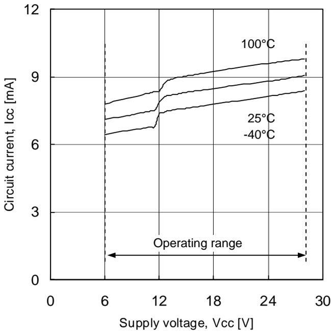
Fig.3 Circuit current
