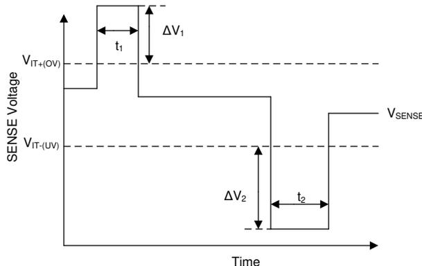
**Figure 8-4. Overdrive Voltage on the SENSE Pin**
