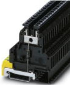
Modular terminal block with suppressor diode as surge voltage protection between clamping connector and DIN rail, separate ground connection, nominal voltage: 12 V DC, mounting on NS 35/7.5, terminal width: 6.2 mm, terminal height: 69 mm
