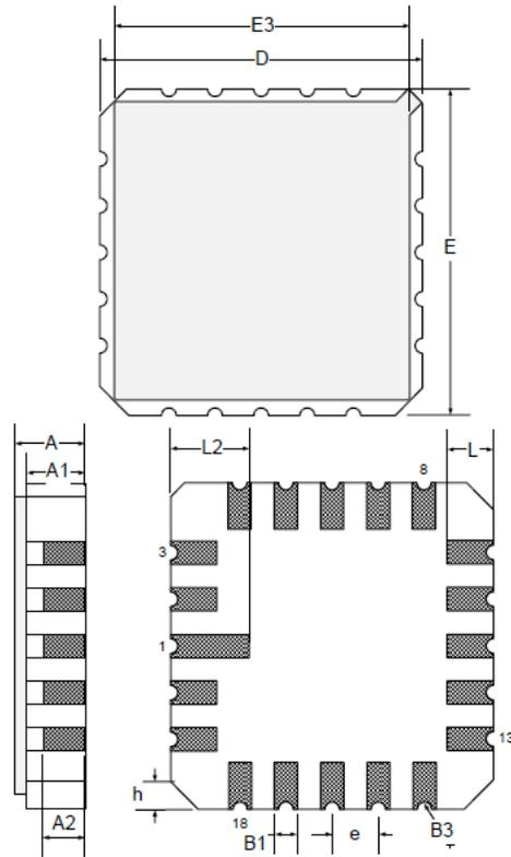
**Table 7 • L 20-Pin Ceramic Leadless Chip Carrier (LCC) Package Outline Dimensions**
