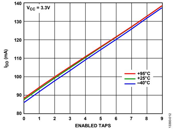
Figure 13. Supply Current vs. Enabled Taps Over Temperature
