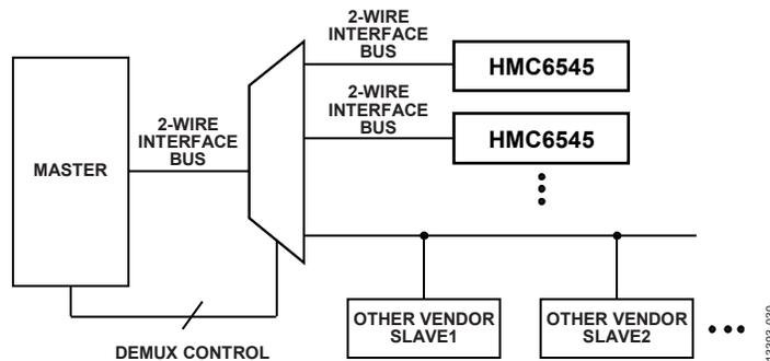
Figure 33. Multiple HMC6545 Devices on 2-Wire Interface Bus
