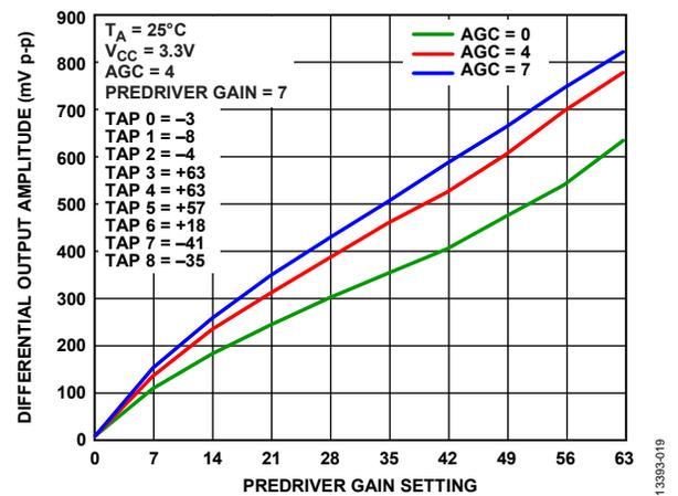
Figure 20. Differential Output Amplitude vs. Predriver Gain Over AGC, Input Signal: Differential PRBS 2<sup>31</sup> - 1, 10 Gbps at 500 mV p-p
