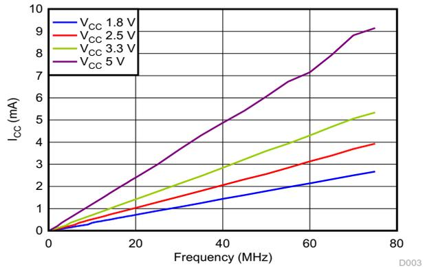
Figure 9-2. I<sub>CC</sub> vs Frequency
