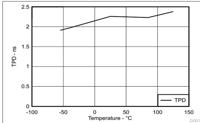
Figure 6-1. TPD Across Temperature at 3.3 V<sub>CC</sub>
