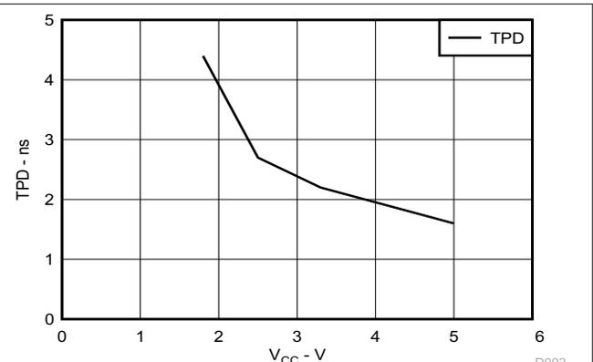
Figure 6-2. TPD Across V<sub>CC</sub> at 25°C
