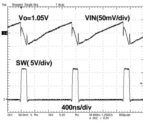
Figure 15. VOLTAGE RIPPLE AT INPUT (IO = 6 A)
