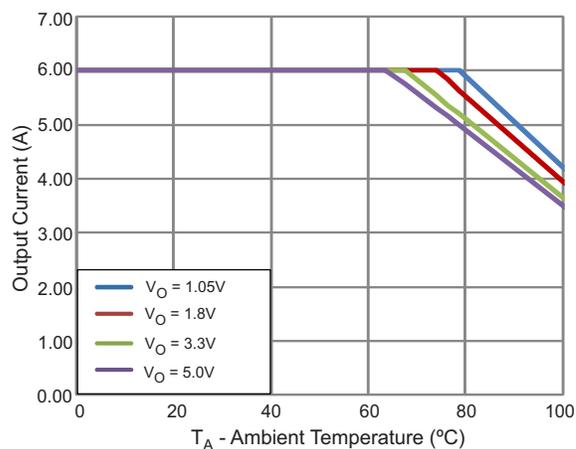
Figure 16. OUTPUT CURRENT vs AMBIENT TEMPERATURE
