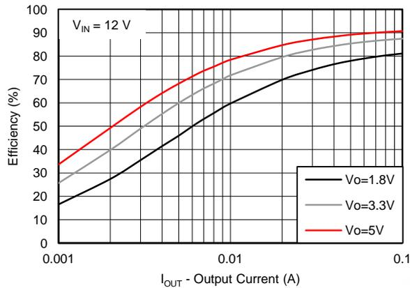
Figure 9. LIGHT LOAD EFFICIENCY vs OUTPUT CURRENT
