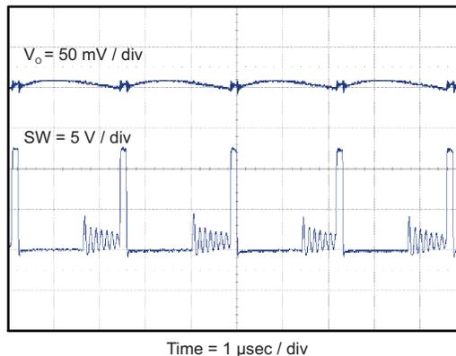
Figure 14. DCM VOLTAGE RIPPLE AT OUTPUT (IO = 30 mA)
