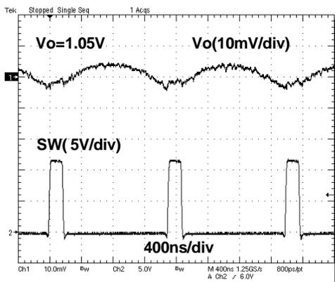
Figure 13. VOLTAGE RIPPLE AT OUTPUT (IO = 6 A)
