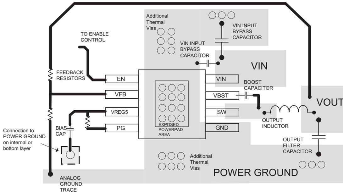
**Figure 19. PCB Layout**
