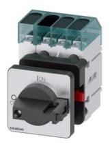
Load disconnector 3LD3, lu 40 A Main switch 3-pole + N Rated operating capacity at AC-23 A at 400 V 18.5kW Front plate mounting Basic switch with Central hole mounting 22.5mm Toggle drive black 48x48 mm
