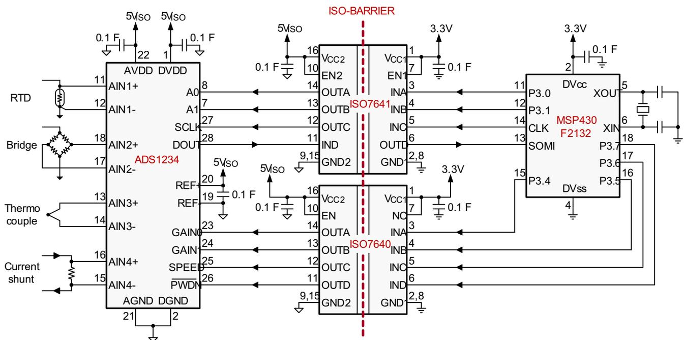
Figure 16. Isolated Data Acquisition System for Process Control
