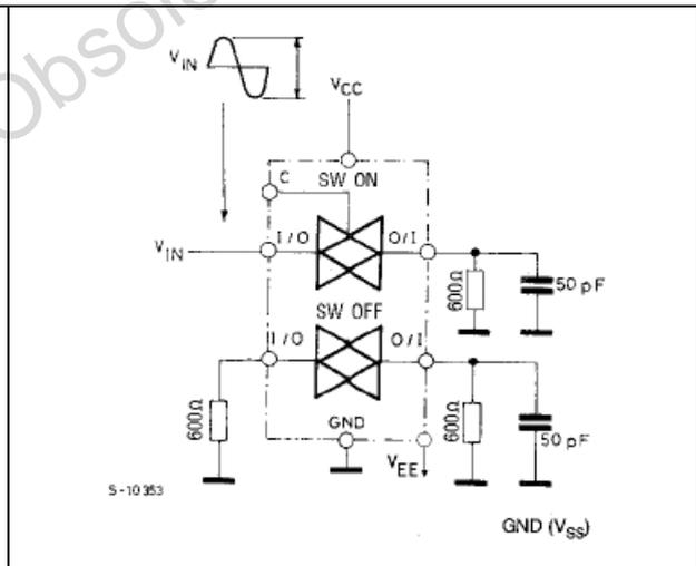
Figure 10. Common terminal capacitance ( $C_{I-O}$ ,  $C_{I/O}$ )
