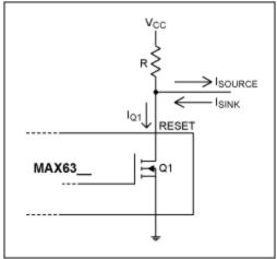
Figure 1. Open-drain output.
