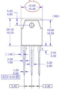
Description of Change (To) : Heat sink width drawing spec: 15.40-16.20mm
