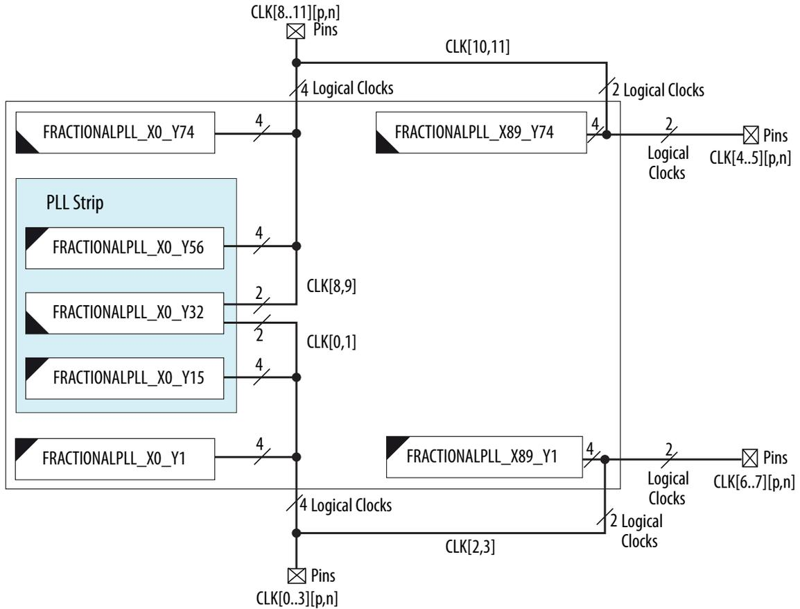
**Figure 4-20: PLL Locations for Cyclone V E A9 Device, Cyclone V GX C9 Device, and Cyclone V GT D9 Device**
