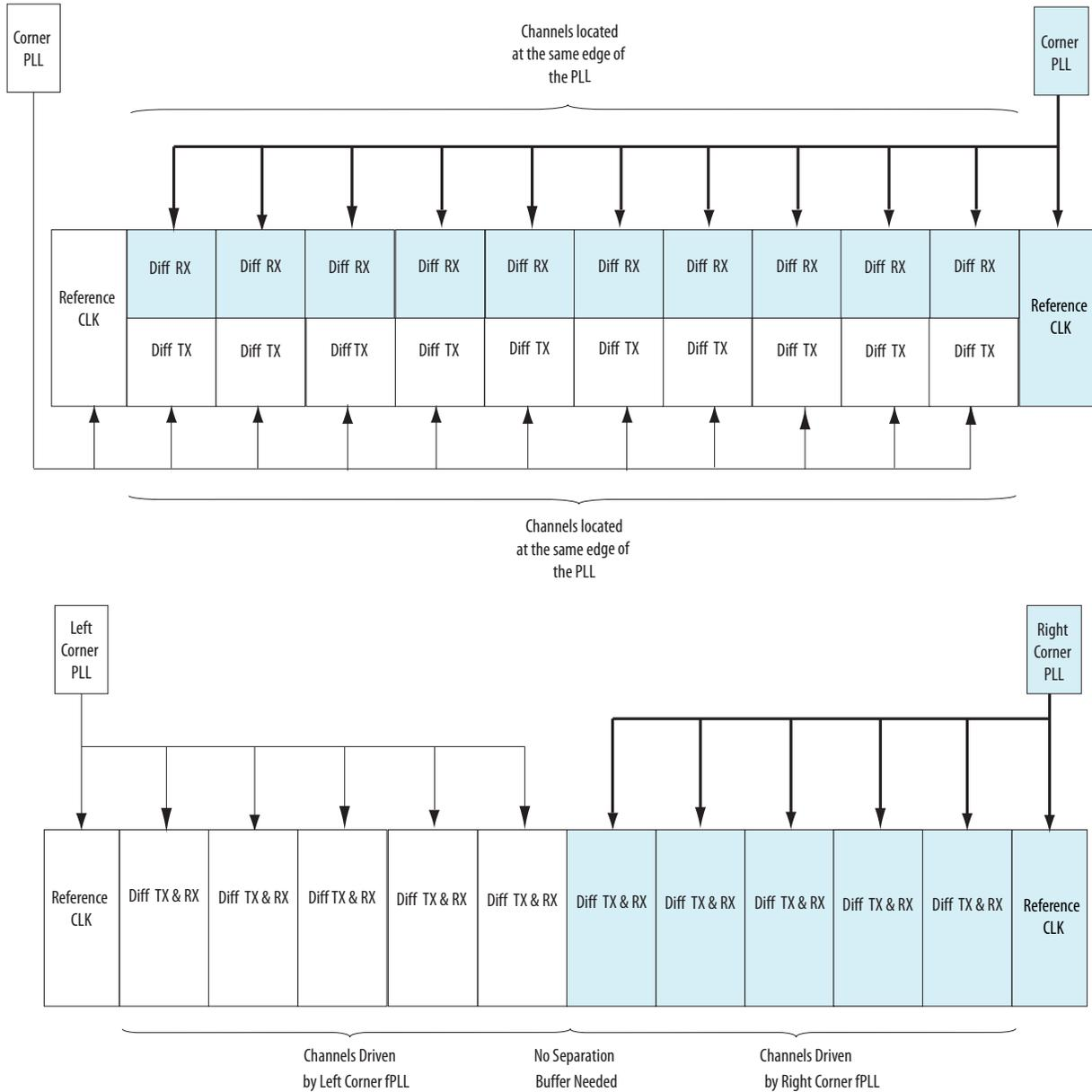
**Figure 5-3: Invalid Placement of Differential I/Os Due to Interleaving of Channels Driven by the Corner PLLs**
