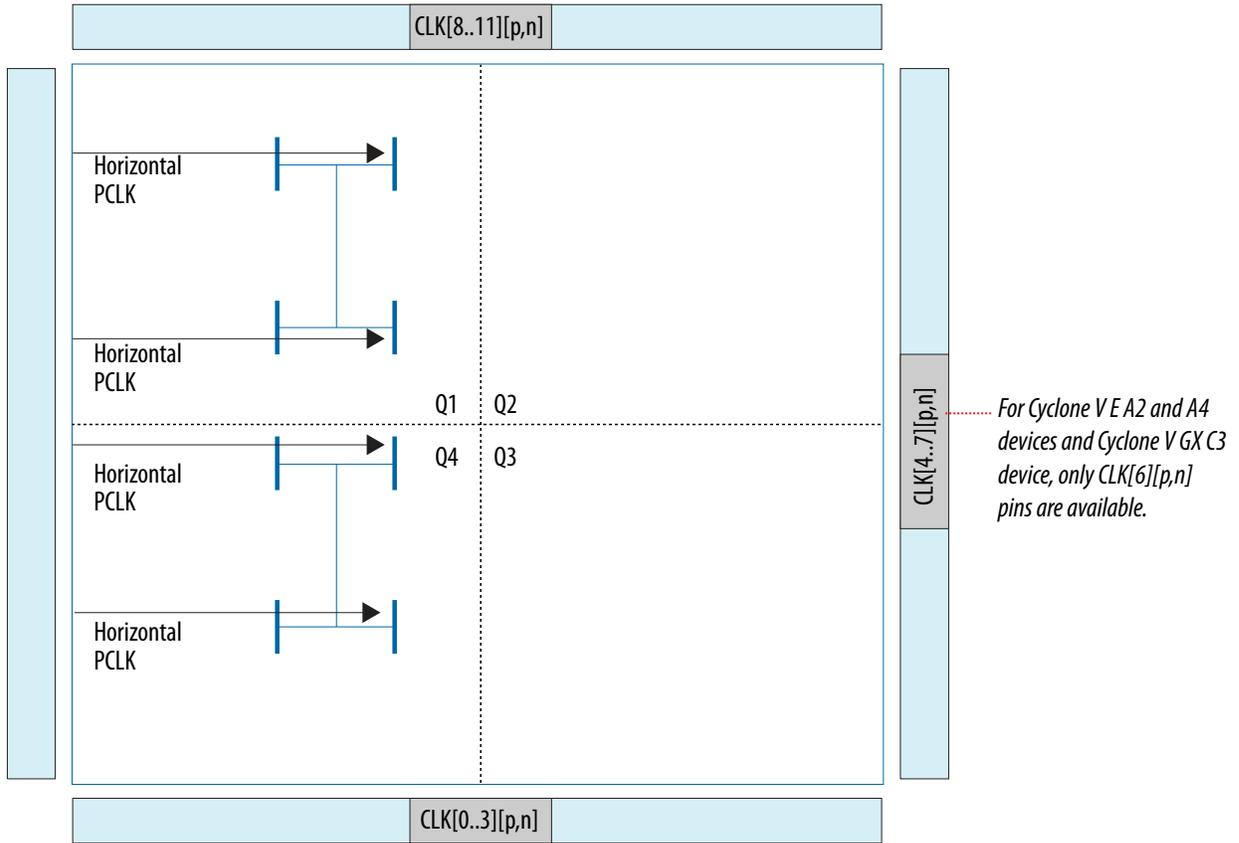
**Figure 4-6: PCLK Networks in Cyclone V SE, SX, and ST Devices**
