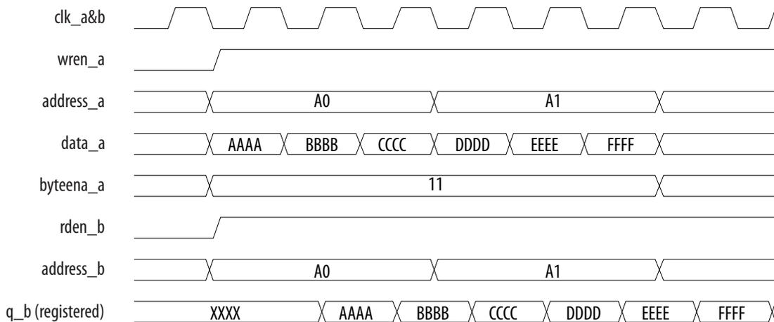
**Figure 2-4: Mixed-Port Read-During-Write: Old Data Mode**
