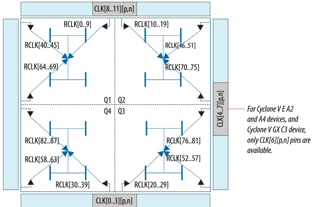
**Figure 4-4: RCLK Networks in Cyclone V SE, SX, and ST Devices**
