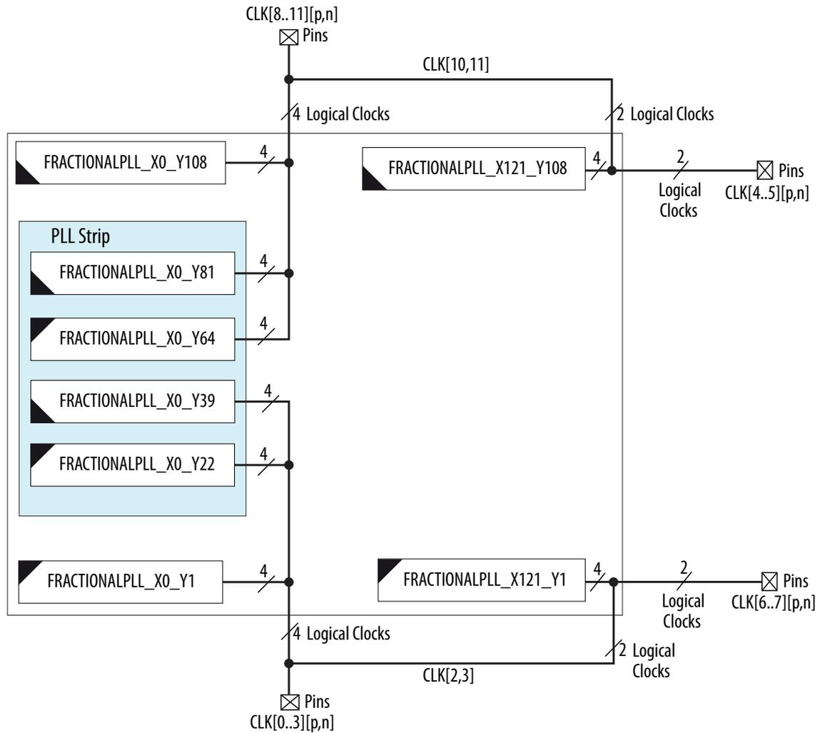
**Figure 4-21: PLL Locations for Cyclone V SE A2 and A4 Devices, and Cyclone V SX C2 and C4 Devices**
