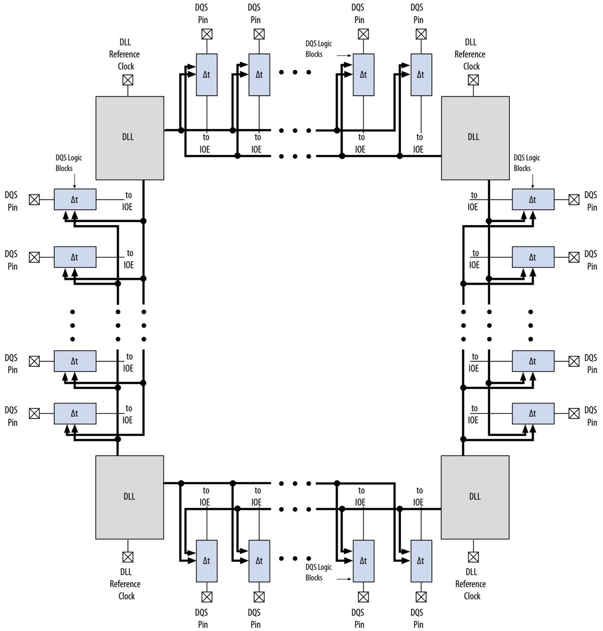
Figure 6-3: DQS Pins and DLLs in Cyclone V GX (C3) Devices
