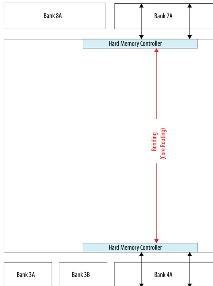
**Figure 6-24: Hard Memory Controllers in Cyclone V SX C2, C4, C5, and C6 Devices, and Cyclone V ST D5 and D6 Devices**
