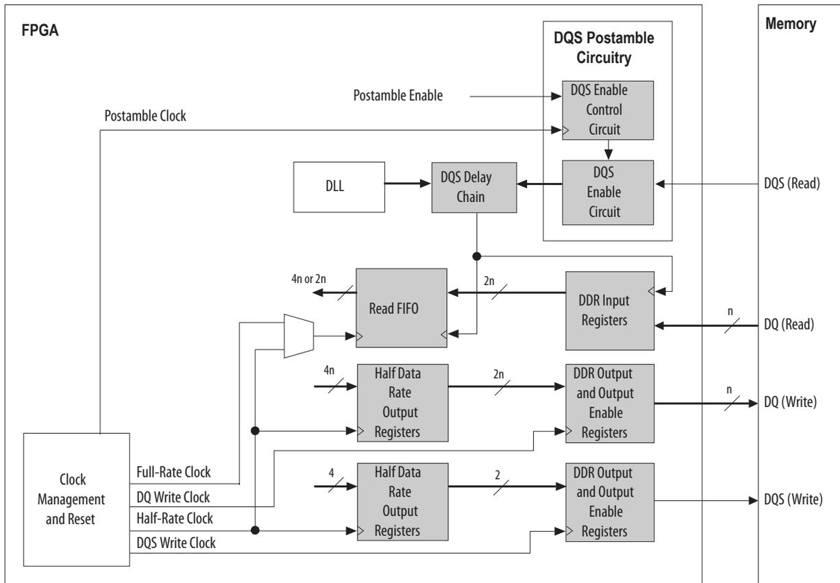
**Note:** There are slight block differences for different memory interface standards. The shaded blocks are part of the I/O elements.
