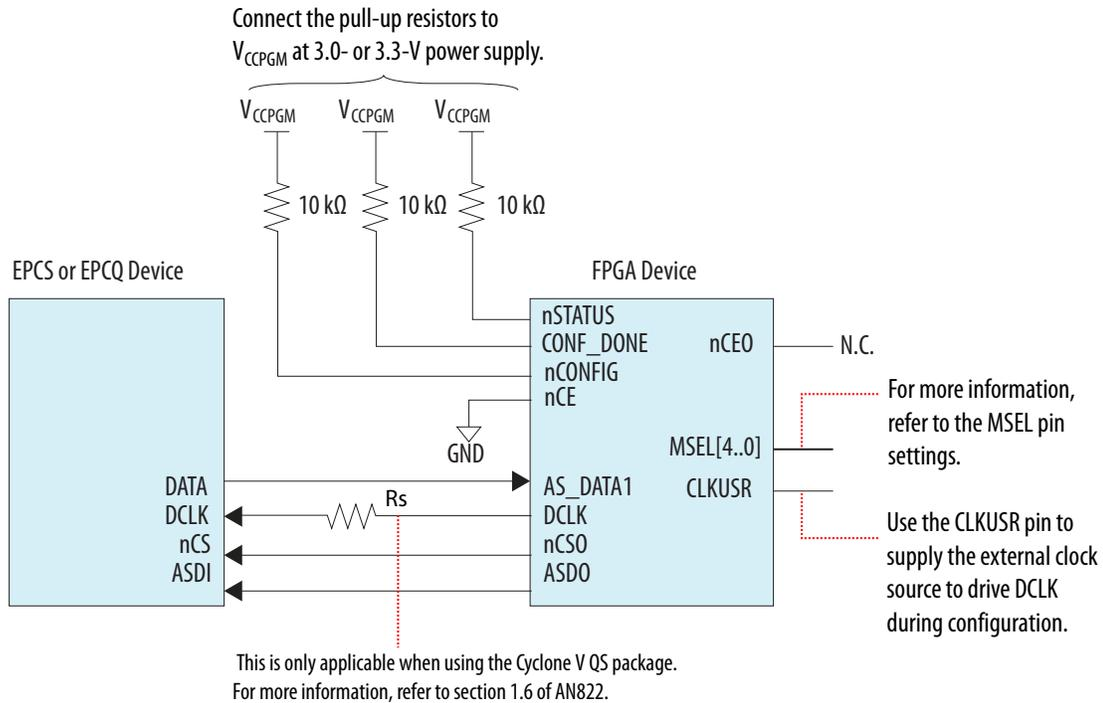
Figure 7-10: Single Device AS x4 Mode Configuration
