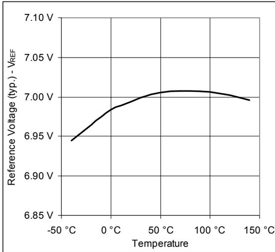
**Fig. 5 - Reference Voltage**
