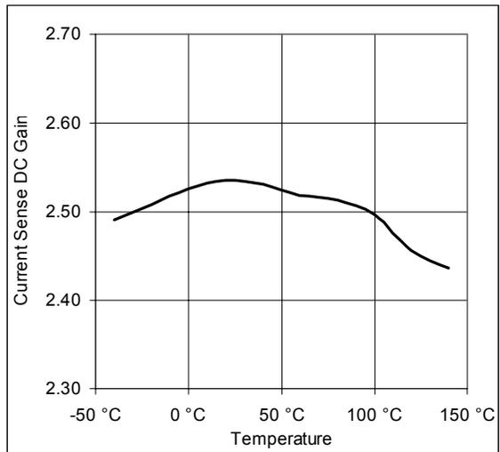
**Fig. 8 - Current Sense Amplifier DC Gain**
