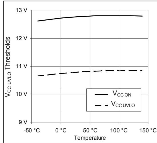
**Fig. 2 - Under Voltage Lockout vs. Temperature**
