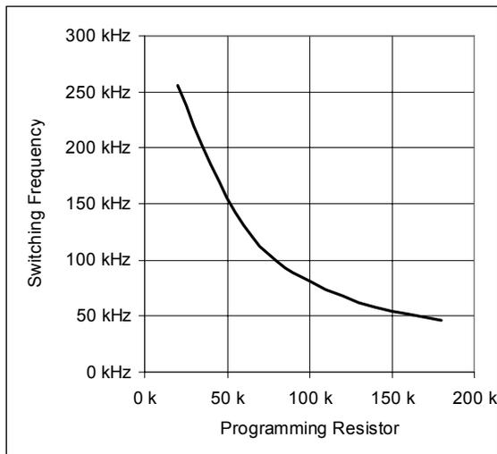
**Fig. 3 - Oscillator Frequency vs. Programming Resistor**
