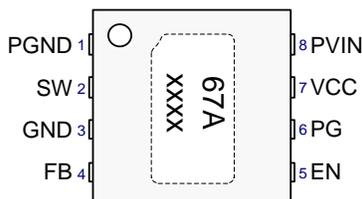
Figure 2 · Pinout DFN 2mmx2mm 8L Top View
