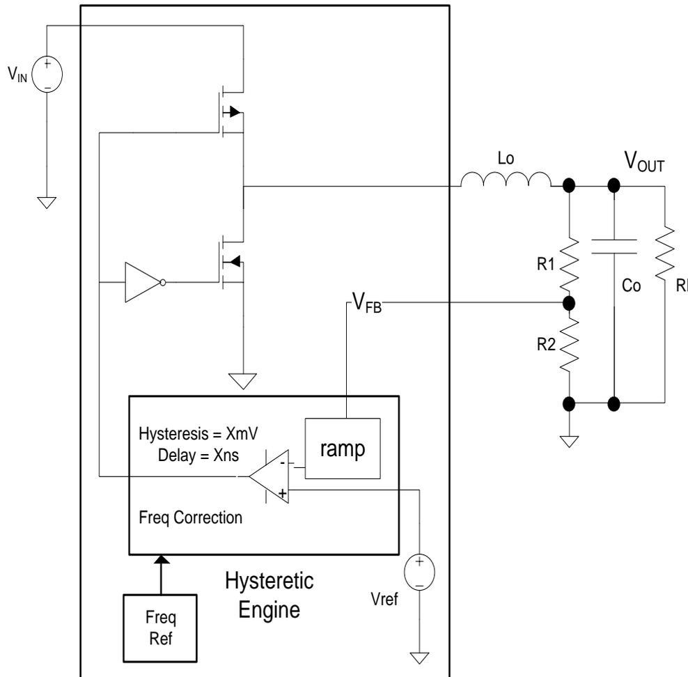
Figure 3 - Simplified Block Diagram of LX7167A
