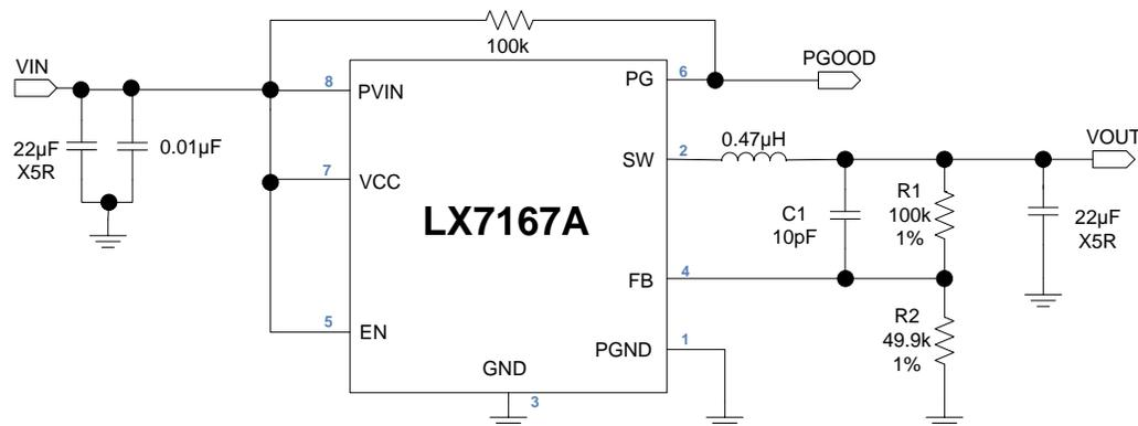
Figure 7 · LX7167A Typical Application Diagram
