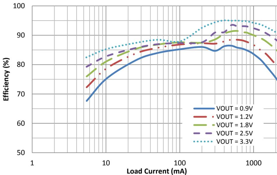
Figure 5 · Efficiency vs. Output Current with 5V Input
