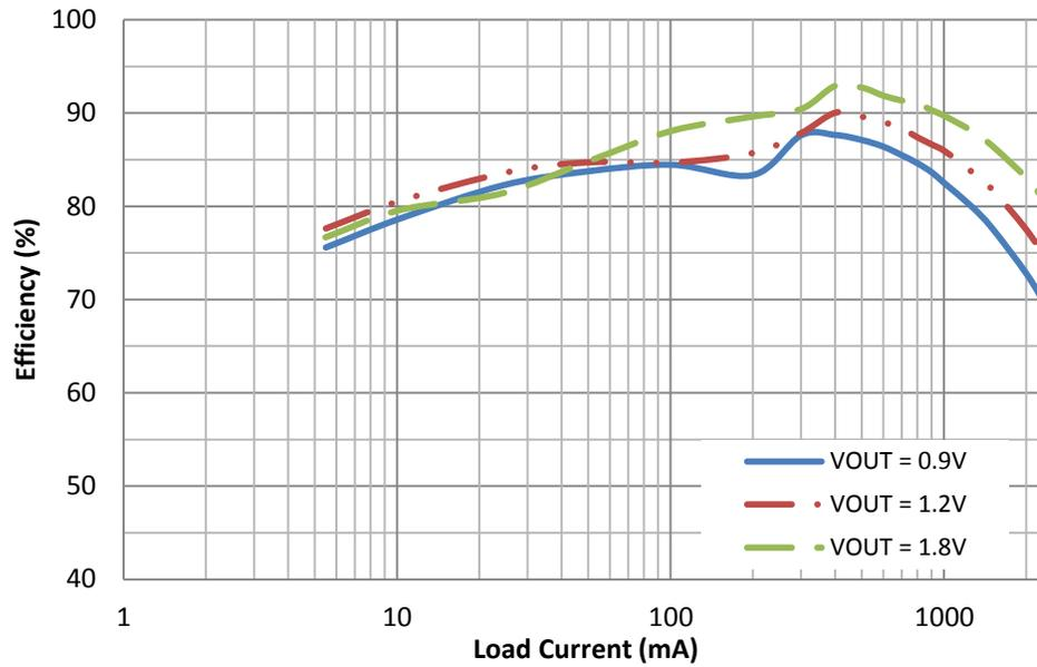
Figure 4 · Efficiency vs. Output Current with 3.3V Input
