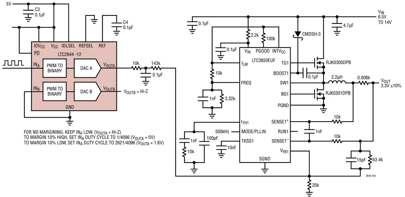
Figure 4. Voltage Margining Application with LTC3850 (3.3V ±10%)
