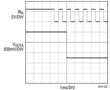
**Exiting Idle Mode Power-Down (1 Channel) to Mid-Scale (IDLSEL =  $V_{CC}$ )**
