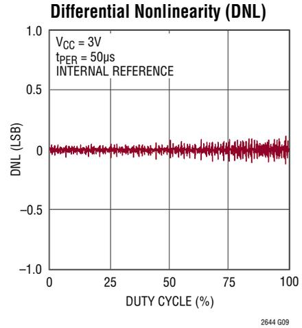
**LTC2644-8 (Internal Reference,  $V_{FS} = 2.5\text{V}$ )**
