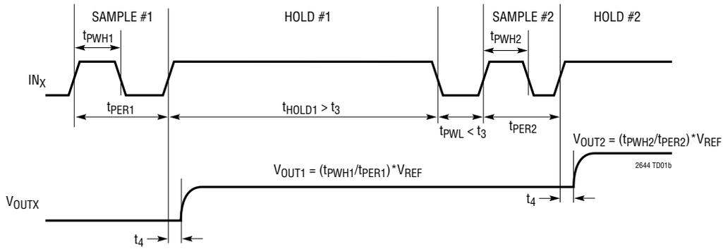
**Figure 1b. Sample/Hold Operation (IDLSEL = V<sub>CC</sub>)**
