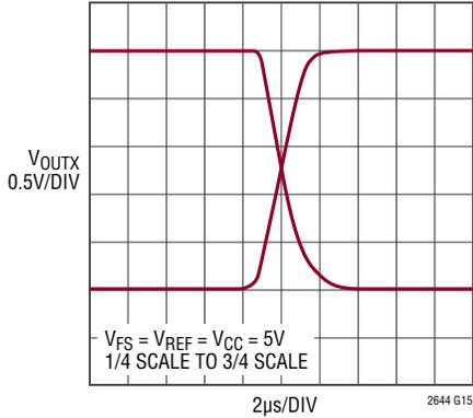
**$IN_X$  to  $V_{OUTX}$  Delay Full-Scale Transition**
